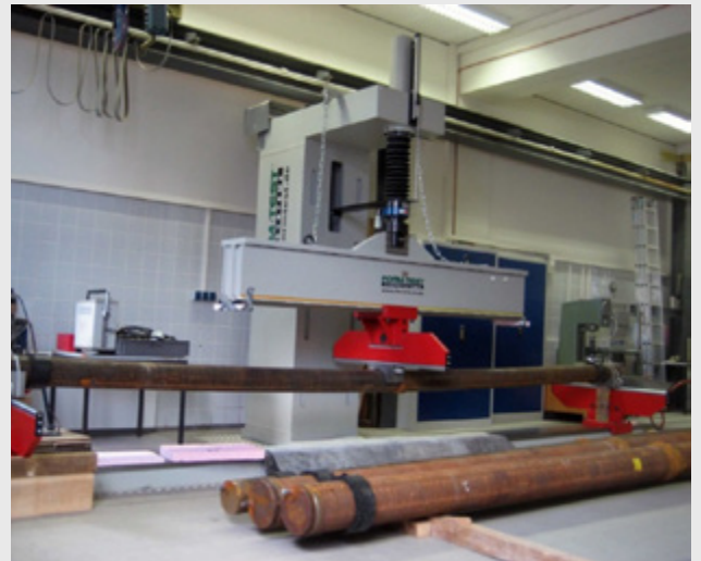
Figure 4: Test portal for bending tests (manufacturer: FORM+TEST, Riedlingen, Germany)
