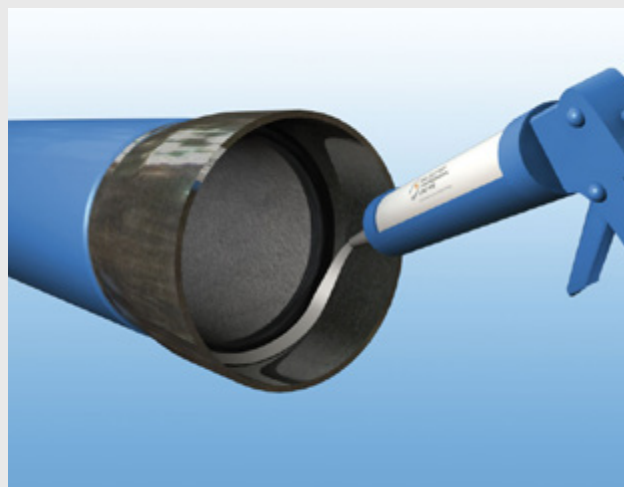
Figure 2: Sealant application to the socket base before welding
