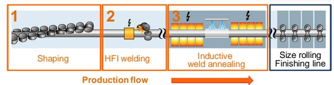
Figure 1: Pipe production via HFI-process (schematic)
