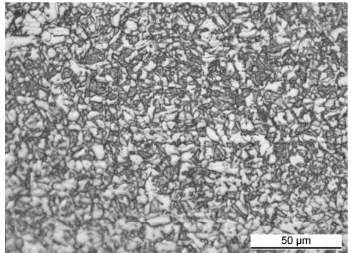
Figure 4: Microstructure of base material after Q&T-process
