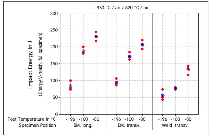
Figure 6: Impact energy after Q&T-processing as a function of test temperature and specimen positioning
