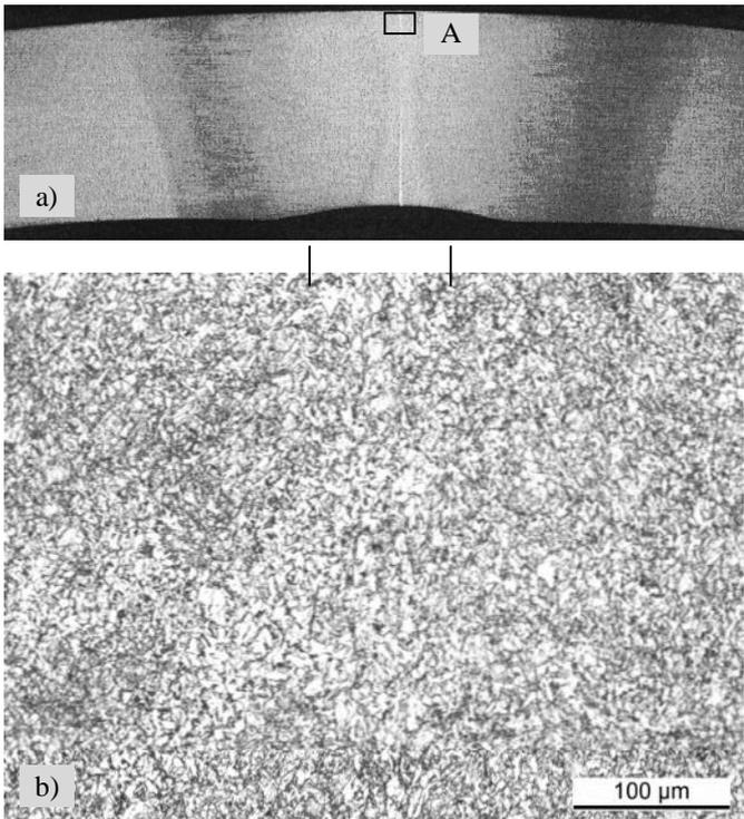
Figure 5: Microstructure of HFI-weld area after Q&T-process with b) as enlargement of position A in a) and marking of fusion line width in b)
