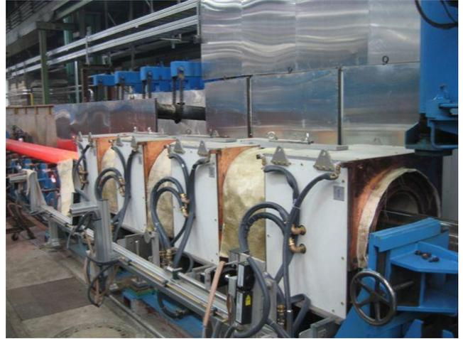
Figure 3: Pipe during full-body annealing
