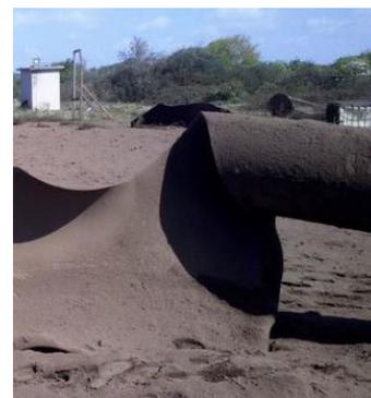
Burst test on a CO<sub>2</sub> test line. CO<sub>2</sub> mixture ( 94.0% CO<sub>2</sub> ) at 127 bar, material X65, measuring 610 x 13.7 mm, from the RFCS-funded SARCO2 project. Cracking in the steel pipe is arrested after a few meters.
