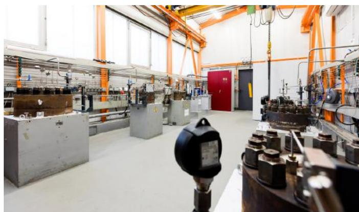
Test setup for CO<sub>2</sub> corrosion tests (rotating cage) and autoclave laboratory at Salzgitter Mannesmann Forschung GmbH
